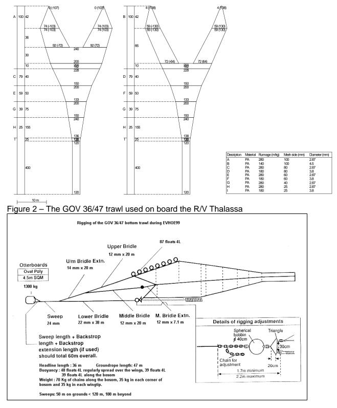
Figure.3 Rigging of GOV 36/47 used during EVHOE surveys
