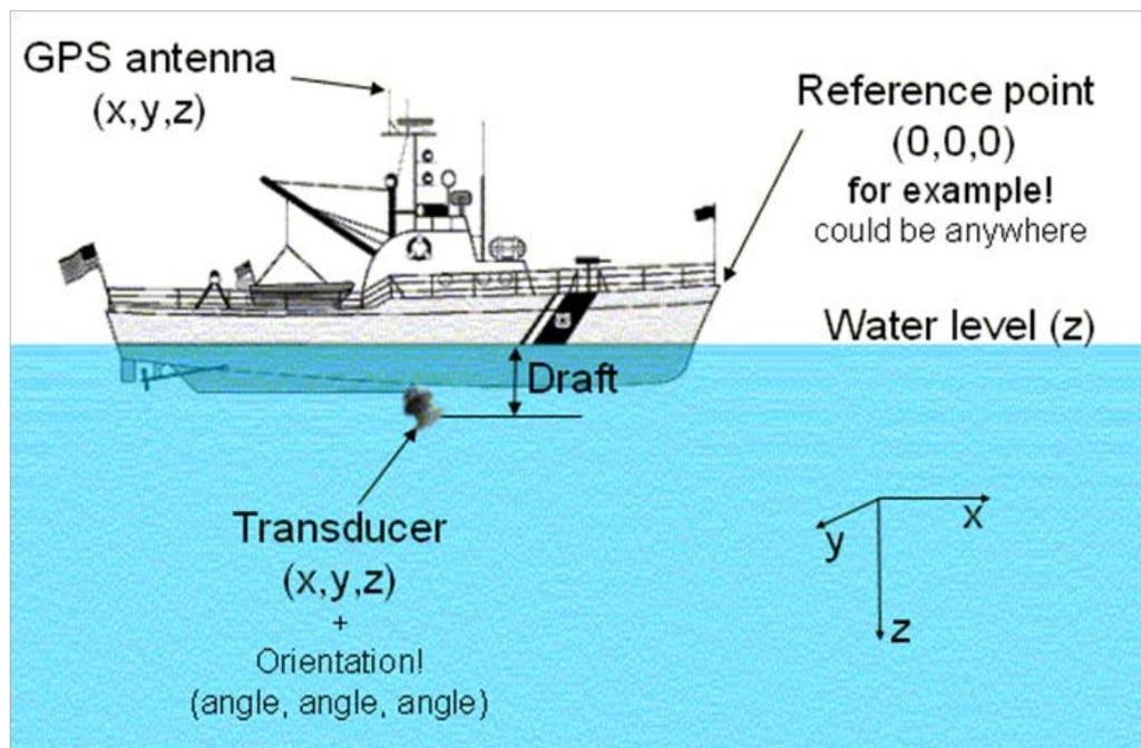
Transducers are always associated with a platform. The reference point of the platform is at (0,0,0) by definition and defines the position of the platform in the real world (that is, the platform is considered to be, in the real world, wherever its reference point is).
