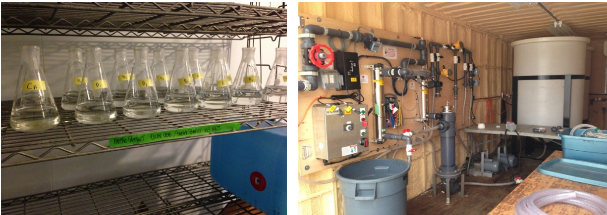
Figure 1. Left) Phytoplankton cultures with chlorine treatments; Right) Shore-side testing lab with filter + UV lamp.
