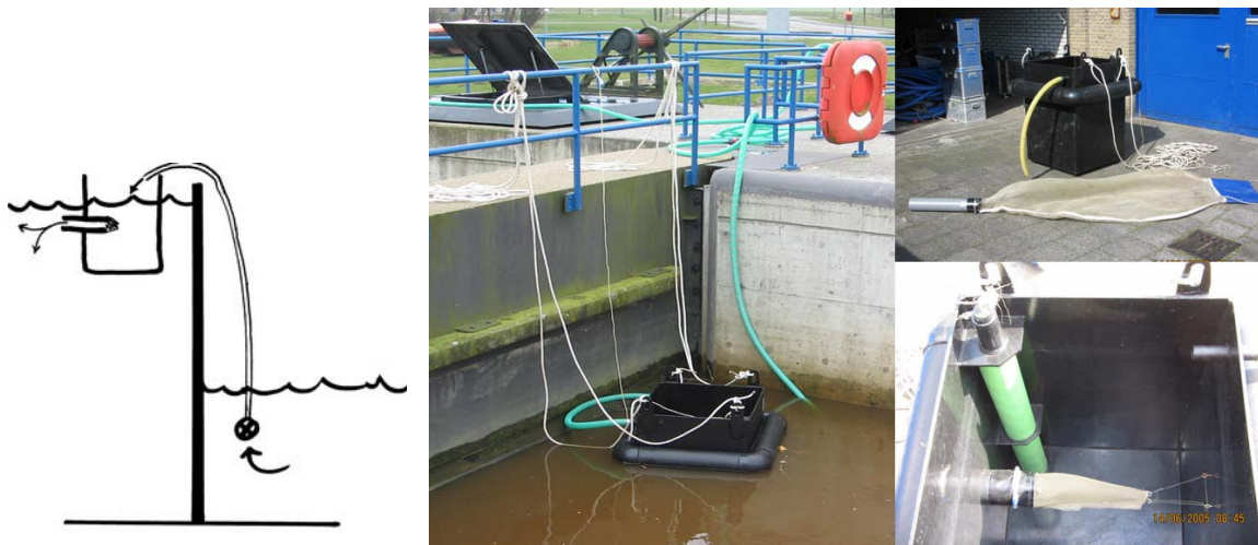
Figure 3. Eel trap at high tide. Arrows indicate the direction of the water flow through the trap.
