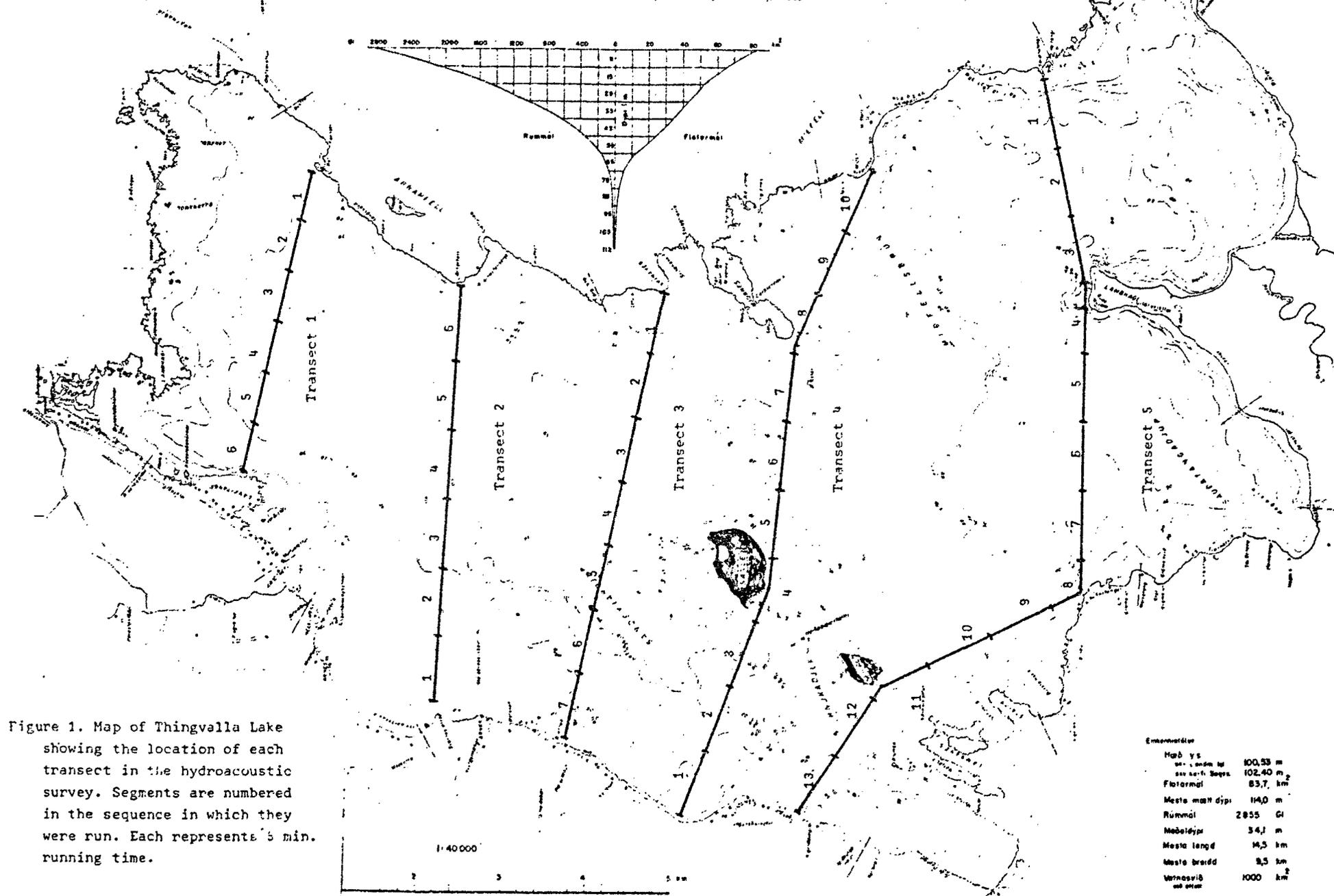
Figure 1. Map of Thingvall Lake showing the location of each transect in the hydroacoustic survey. Segments are numbered in the sequence in which they were run. Each represents 5 min. running time.
