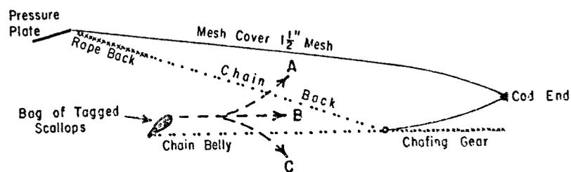
Fig. 2. Diagrammatic vertical section through covered offshore dredge showing method of release of tagged scallops and possible escape routes:
