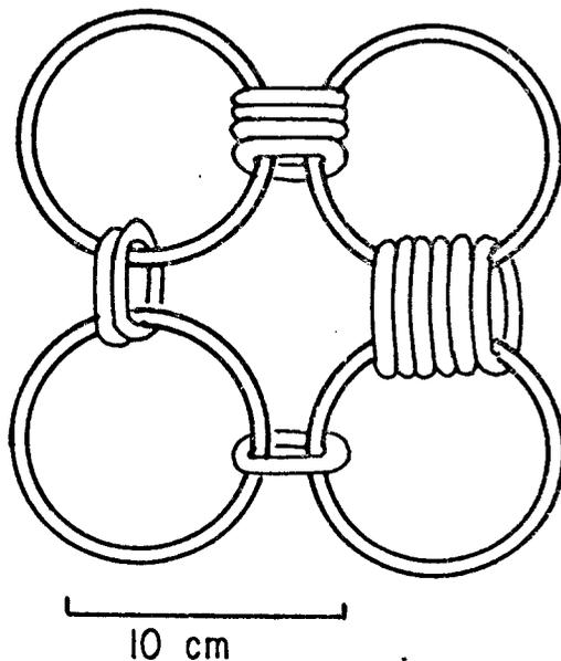
Fig. 4. Canadian offshore scallop dredge ring linkage with 1-6 links per ring.
