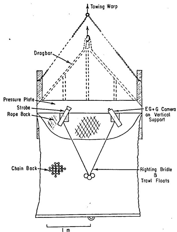
Fig. 1. Canadian offshore dredge showing modifications for use with EG & G Camera. (Shaded areas: additions to dredge; dashed outlines: deletions).
