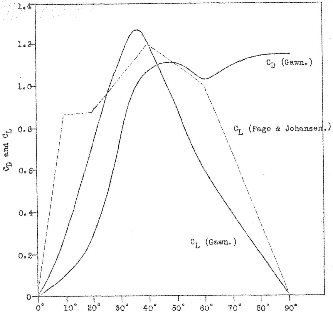
Fig. 8. Lift and Drag Coefficients for flat plates.
