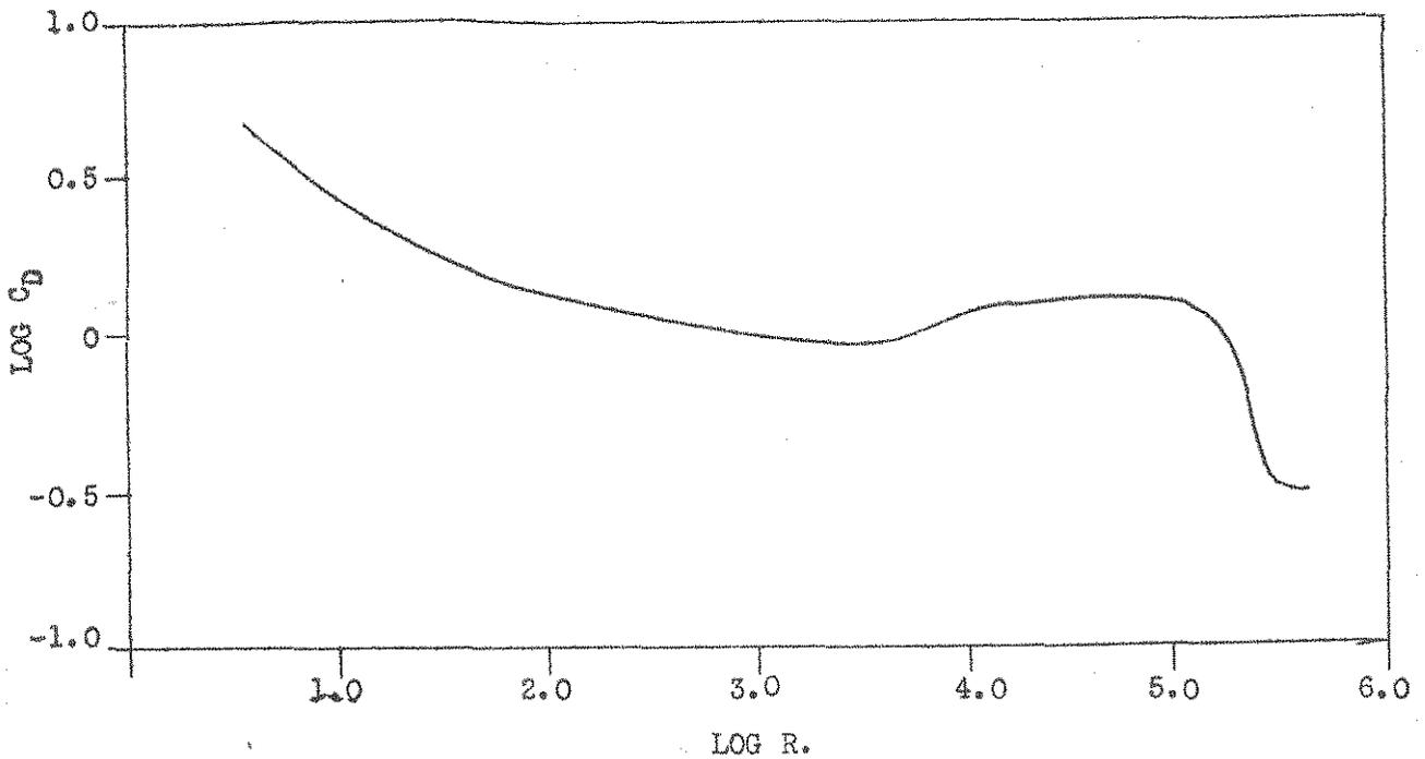
Fig. 12. Change of drag coefficient with Reynold's number.
