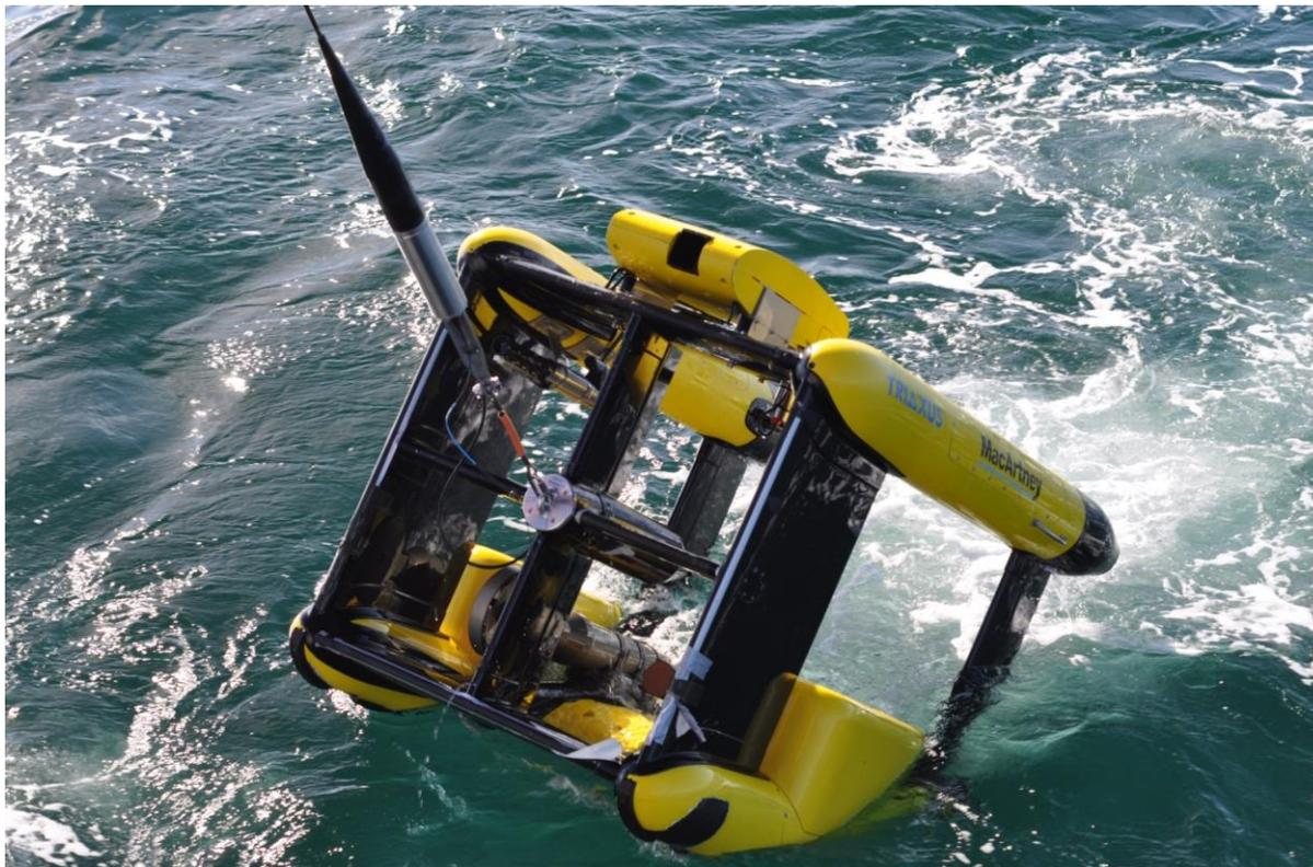
**Scientific equipment** connected via fibre optic cable (2000m)
