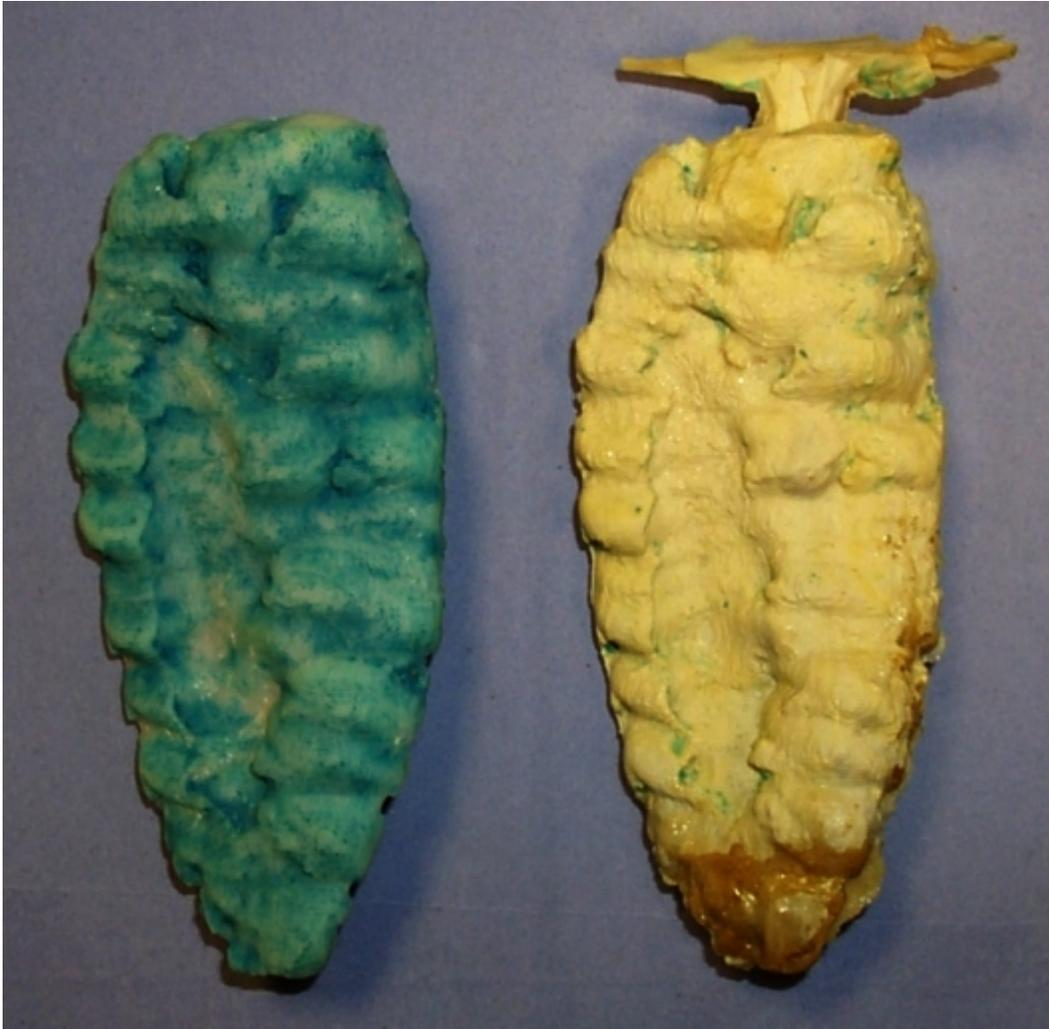
**Figure 5.108:** The original prototype (left) and the replica (right) are shown. The colors are due to the colored synthetic clay and other effects. After removal of the cast-hole parts, finishing the final model is advised.
