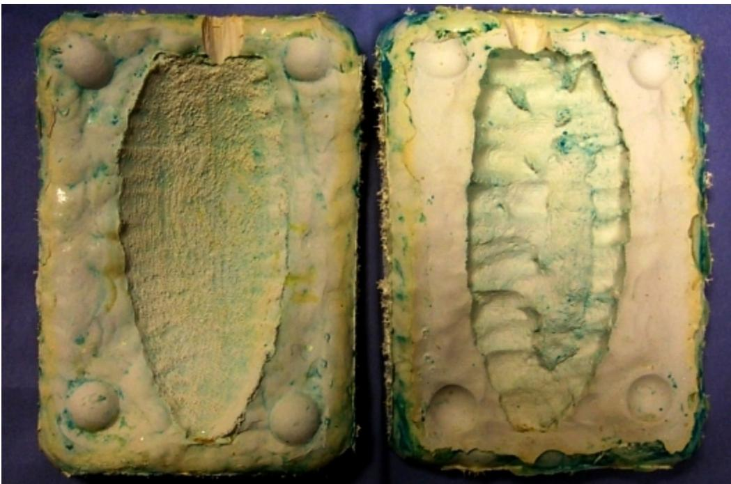
**Figure 5.107:** This image shows the two halves of the latex cast. An opening has been carved at the top sides of the two halves for pouring in the Alumilite. Half-spherical protrusions are visible at the four corners of the left cast, with corresponding impressions on the right cast - these are used for aligning the halves to one another and locking them into position.
