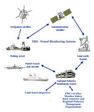
Figure 7. The principles for the VMS system. Source: http://ec.europa.eu/
