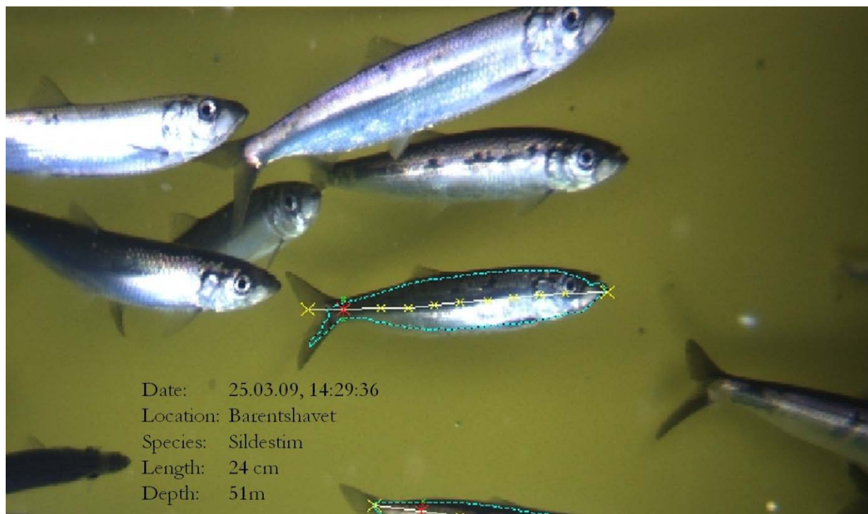
Figure 8 - Fish size and species (herring) identified in situ by stereo-optic measurements (Photo: Scantrol AS).
