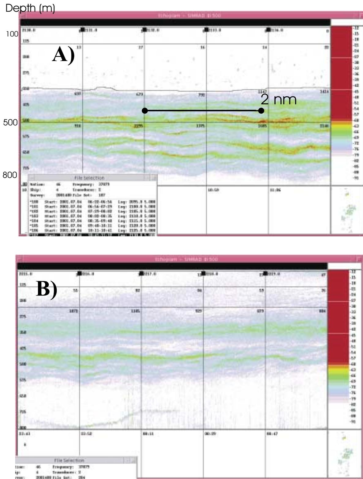
**Figure 2.** Example of echograms obtained during the June/July survey in 2001. The figures is from 3-4. July and figure A) shows registration during daytime (at 55°46N-37°30W, from 10:41-11:06 on 4<sup>th</sup> of July) and B) during dark hours (at 55°45N-40°50W, from 23:43 on 3. July to 00:47 on 4<sup>th</sup>). The figures shows distance of 5 n.m. from 50 m depth down to 850 m.
