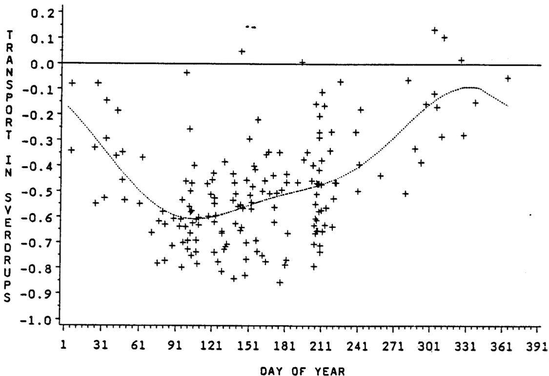
**Fig. 3.** Seasonal cycle of geostrophic transport on the Flemish Cap Line. (a) Transport between stations 2 and 7 over the Grand Banks, and (b) between stations 7 and 14 through the Flemish Pass. Each data point represents the transport calculated for a single transect. The seasonal cycle is shown by the dashed line. Transports calculated for top 100 m.
