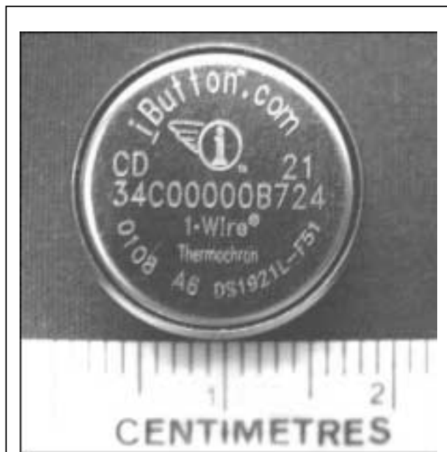
The IButton records only temperature. It is made by Dallas Semiconductor for commercial purposes such as keeping track of ambient temperature of perishable food during transport. Its main advantage is its sale price: 9 $US a piece! We expect resolution of +/- 0.5 to 1°C. IButtons will log a maximum of 2048 points, sampled at a rate of 1 to 255 min. A sample every 4 h will provide a one year time series.
