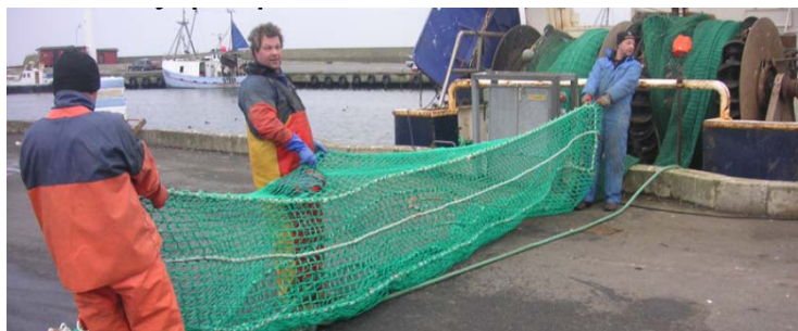
Figure – An 8 m long square mesh side panel codend
