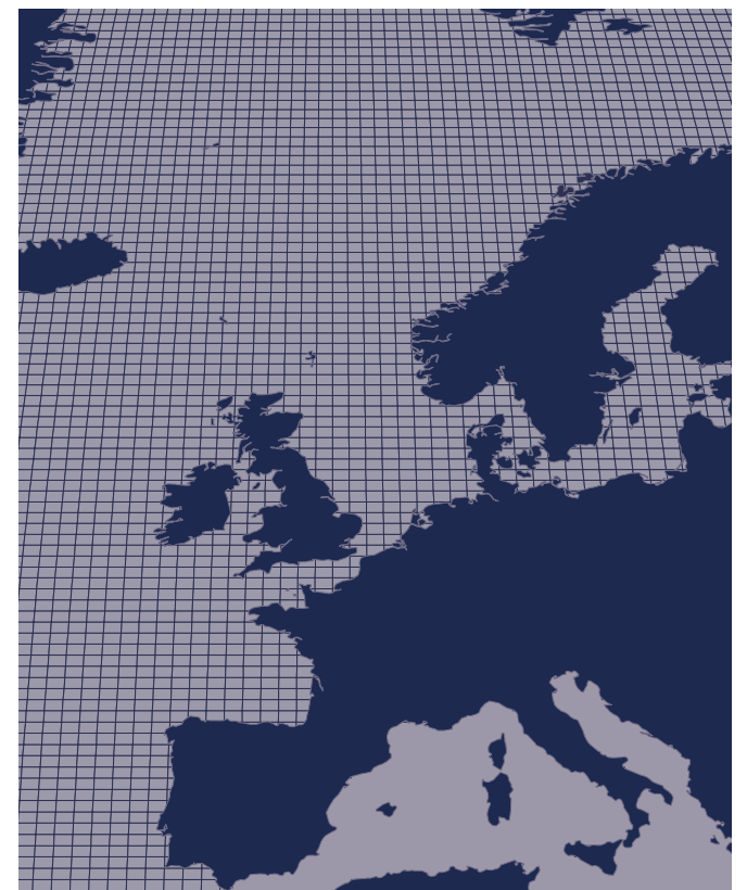
To bring order to the fish-sampling process, ICES divided the Northeast Atlantic into a grid of rectangles of 1 degree of Longitude by 0.5 degrees of Latitude.
