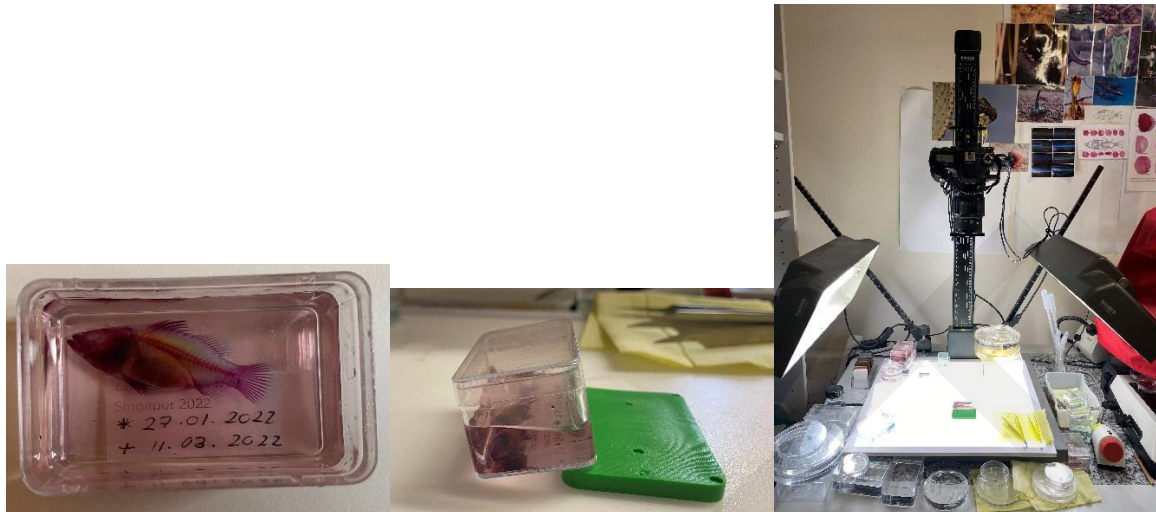
Examples of a specimen in a water filled container, use of moulds to tilt the container to get the specimen flat on the image, and photographing setup with lighting.
